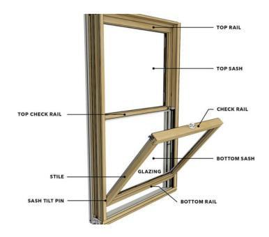
The stationary components of a window that enclose either the sash on an operating window or the glass on a direct glazed window are called the frame. Jambs, sills, and moldings are the primary components of a window frame.
